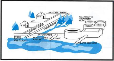
Stormwater flows into the stormwater system through a storm drain. These are frequently located along the curbs of parking lots and roadways. The grate that prevents larger objects from flowing into the storm sewer system is called a catch basin. Once below ground, the stormwater flows through pipes which lead to an outfall where the stormwater enters a stream, river or lake, in most areas of New Jersey, the stormwater sewer goes directly to local waterway without any treatment.
